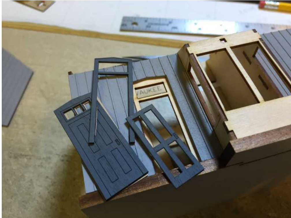
Build the door. There are 5 pieces of the door all double stick except for the glazing.
