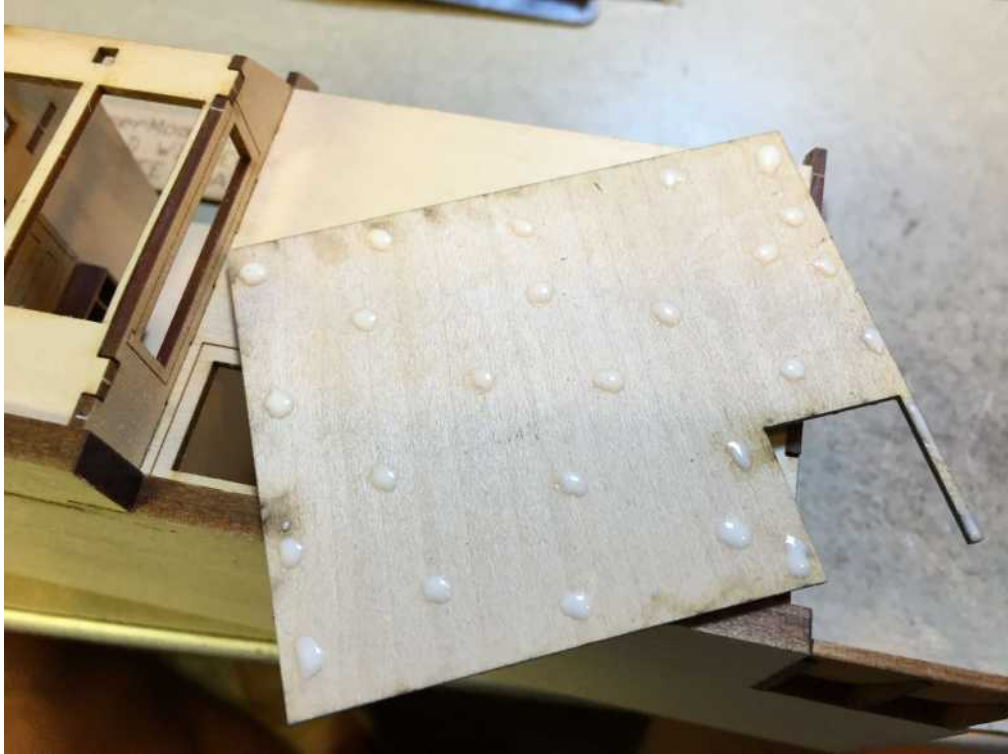
To prevent warping, a few drops will do you when gluing on the siding.
