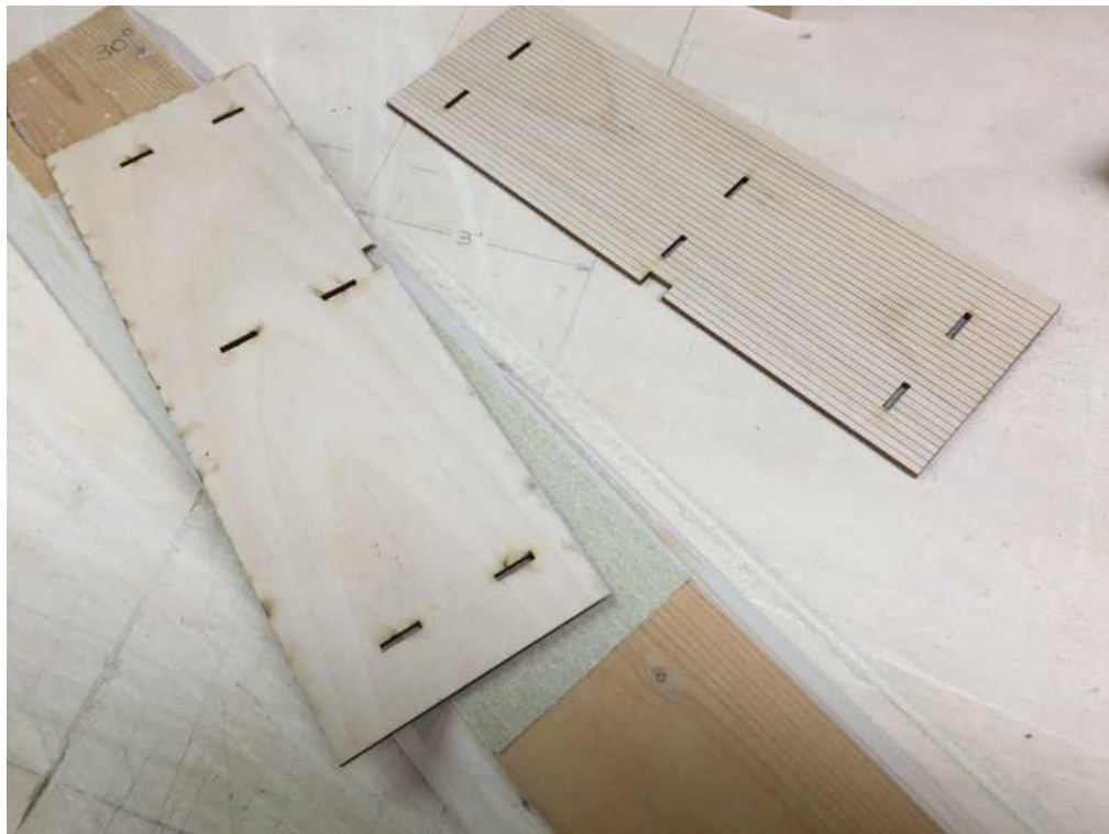
Bevel the roof ridge on each roof piece. The bevel angle is listed on each piece. Bevel from the back.
