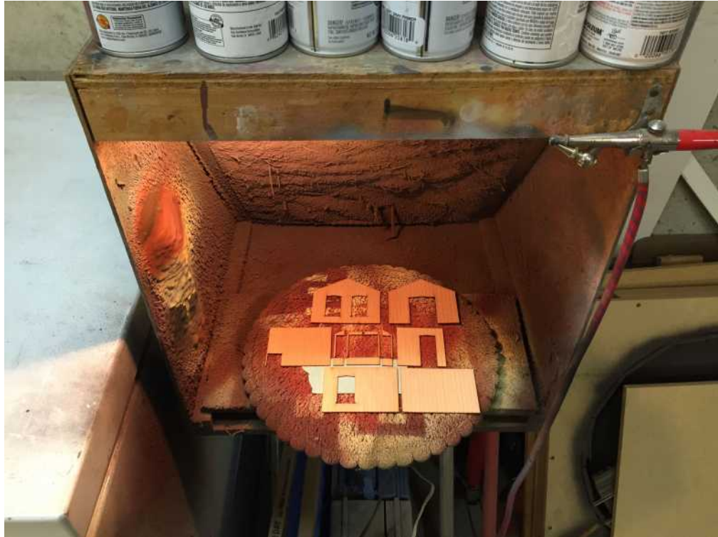
I made a spray paint booth that vents outside with a blower. It has a light and a cake decorating turntable and a changeable furnace filter to knock paint drops out of the air.
