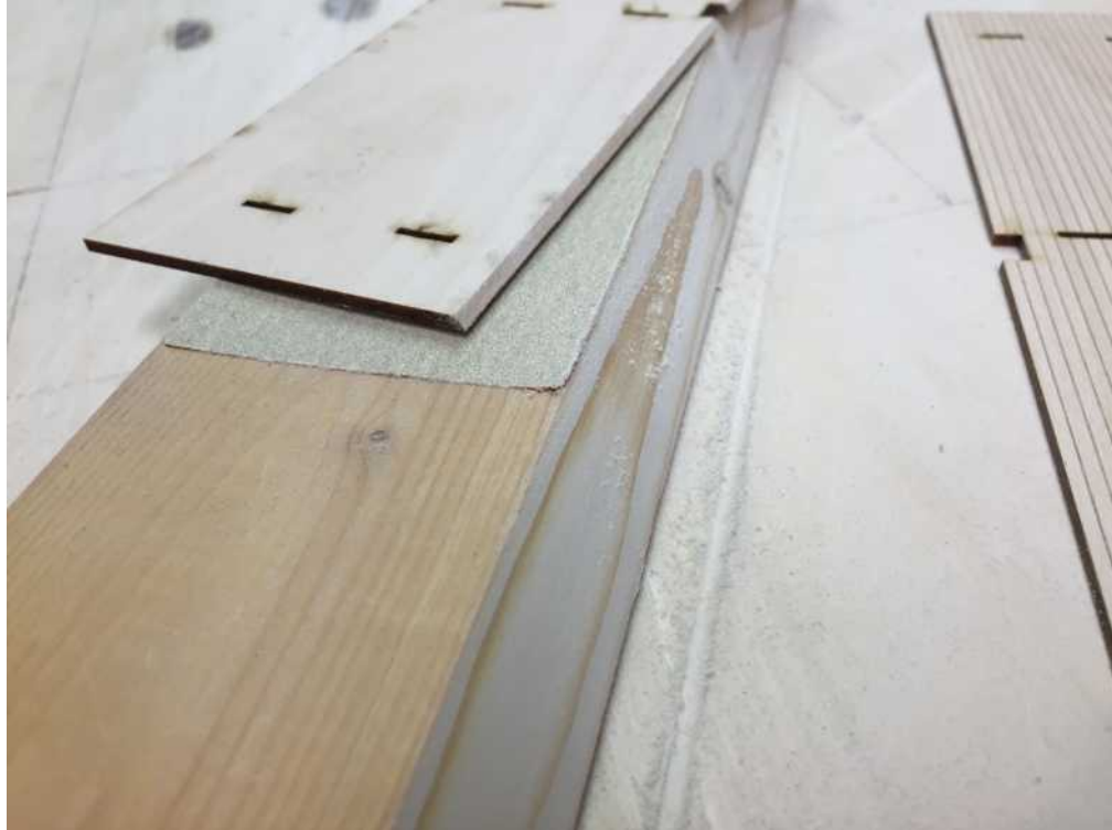
I made some beveling jigs for many different bevels. They are 1"x4" pine with a bevel cut on my table saw. Sandpaper is glued to the top to prevent roof slippage. A sanding block sands the bevel.
