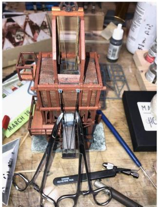
The clamps hold the line taught, I run some CA up and down the line to keep it that way. But as soon as I took off the clamps, static electricity caused the weights to jump and adhere to the bin side, like a magnet!
