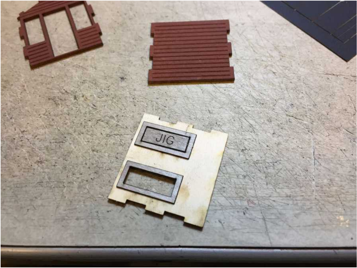
The jig aligns the interior self adhering trim.
