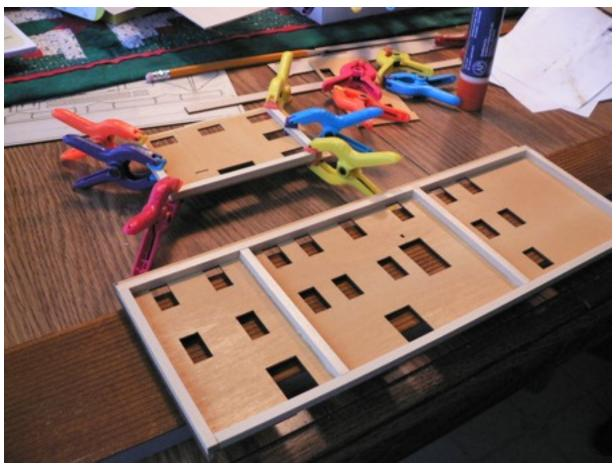
If you model for the outdoors as I also do, warping and dealing with this issue is alway a challenge. The best way to deal with outdoor models is to use only one material for construction. Mixing materials and their different expansion/swelling rates can only lead to warping or adhesive failure.
